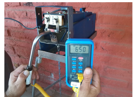
Pyrometer indicating proper blade temperature of 650°C.
